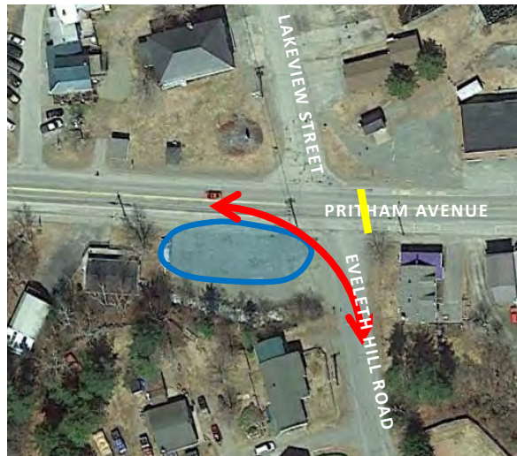
To relieve traffic congestion and the difficult alignment at the intersection of Moosehead Lake Road and Pritham Road - consider realigning the Eveleth Hill Road/Pritham intersection. Additional engineering review required.
