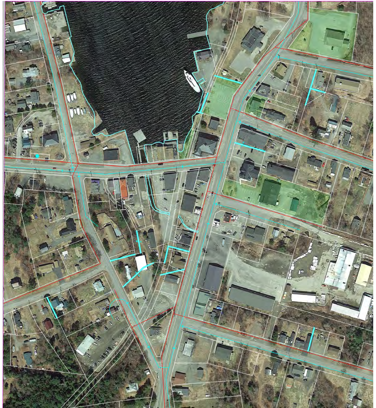
Existing Water and Sewer Lines, Figure 4
